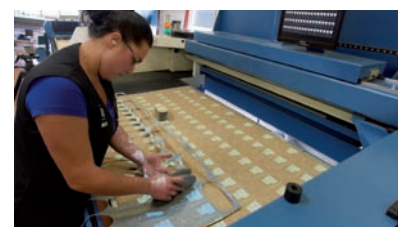
Cutting out foam and resin elements
