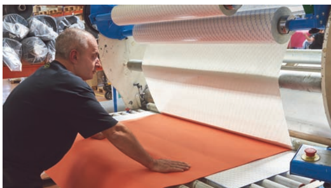
Applying adhesive coating to sheets
