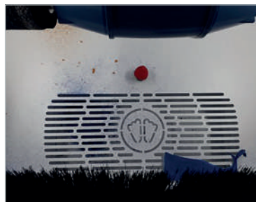
(3) Suction inlet grid designed to facilitate cleaning
